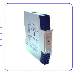
The SEM215 is a universal DIN rail mounted temperature transmitter that accepts most commonly used temperature sensors, slide wire transducers or millivolt signals, isolates and transmits them as a (4 to 20) mA signal to a host system. It can be configured by either of the following methods:
