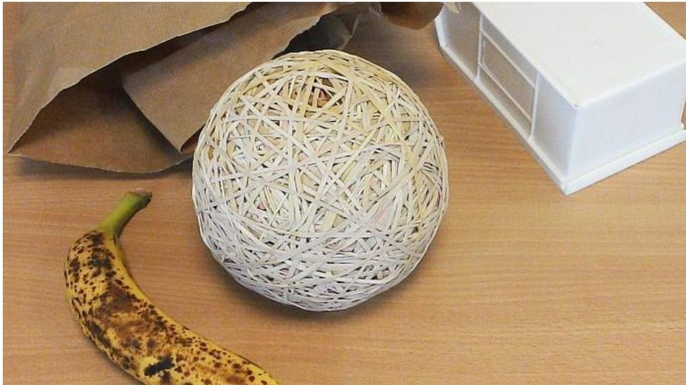
*Examples of materials with high emissivity. Materials like these are easy to measure with general-purpose IR pyrometers.*
