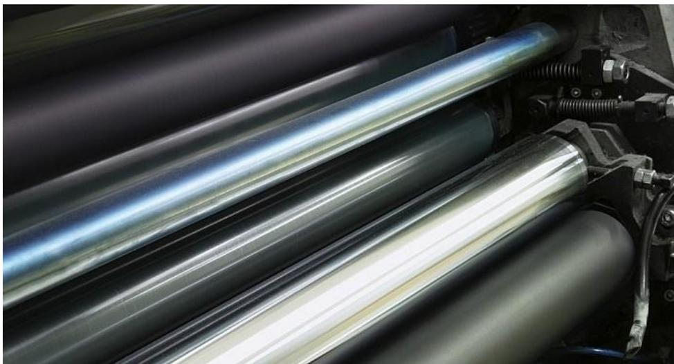
*Reflective metal surfaces are more challenging to measure using infrared temperature sensors. If the surface cannot be painted or coated to make it non-reflective, then a short-wavelength sensor should be used.*
