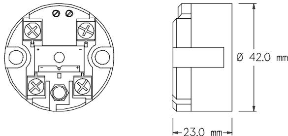
Mounting holes : 2 holes 5.5mm diameter, 33mm centres
