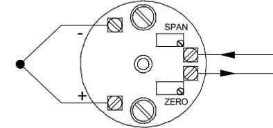
The diagram shows the method of connection to provide a 4-20 mA current loop output.
