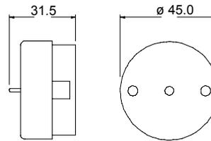
Mounting holes: 2 holes 5.5mm diameter, 33mm centres
