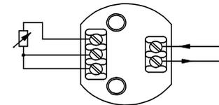
The diagram shows the method of connection to provide a (4 to 20) mA current loop output.
