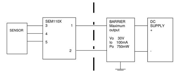
They equipment must be electrically connected as shown below:-
