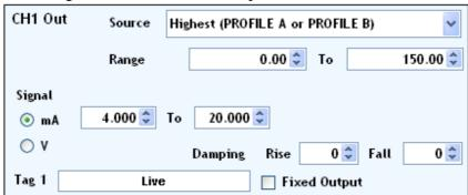
The output for Channel 1 is set to give (4 to 20)  $mA = (0 \text{ to } 150) \text{ }^{\circ}V$ .
