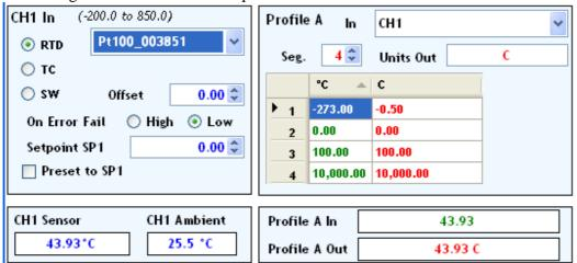
The input probe is a PT100, in the profiling tool input value = output value, apart from -273 °C = -0.5 °C. This in effect will make the profile track the input unless the temperature drops below 0.0 °C or the sensor input is lost (when the external switch is in position 2). At this point the Profile A tool will output -0.5 °C as its value.
