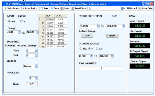
As shown in the data panel the input signal is 18 (18.015). This is giving a process value of 98 (98.02), From the table we see that 18 mA input value = 98 %/R so this is correct.
