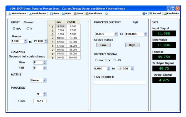
As shown in the data panel the input signal is 12 (11.986). This is giving a process value of 50 (49.75), From the table we see that 12 mA input value = 50 %/R so this is correct.
