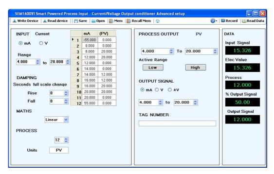
As shown in the data panel the input signal is 15.326. This is giving a process value of 12. From the graph we see that 15.326 mA = 12 PV so this is correct
