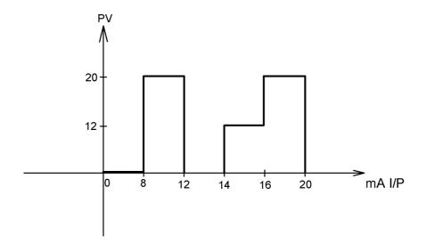
The User Profile Linearization tool can be used in different ways. As well as the examples shown the User Profile Linearization tool can be used to control the way the output responds to **out of range input signals** (see separate instruction).
