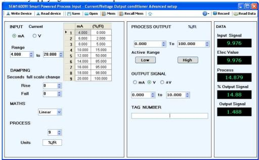
As shown in the data panel the input signal is 10 (9.976). This is giving a process value of 15 (14.88), From the table we see that 10 mA input value = 15 %/R so this is correct
