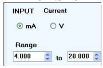
Expand the user profile table to the required number of co-ordinate pairs and enter the data in ascending input order (mA for this example).
