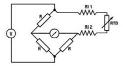
To minimise these errors the three wire compensated bridge was introduced (see figure below).
