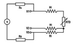
Rc is used solely to limit the current flowing and Rs is a stable reference resistor.
