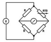
A voltage excites the bridge and the voltage across the bridge is proportional to the resistance of the RTD.
