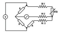
This has the effect of removing the error introduced by the lead resistance as long as lead resistances RL1 and RL3 are matched.
