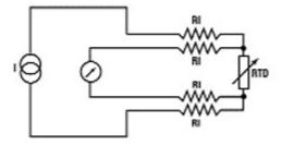
Here the detector is excited by a constant current and the voltage across the detector measured by an amplifier with a high impedance input. If the current source is perfect and the input impedance of the voltage measuring circuit is infinite, then there is no error whatsoever introduced by the lead resistances even if they are mismatched.
